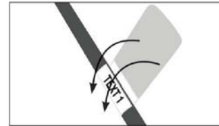
3. Wrap so that white printable area overlaps itself, then continue wrapping clear tail around label
